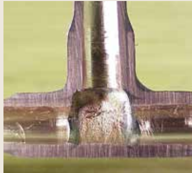
Copper tubing brazed with nitrogen purge.
