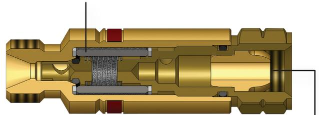
Reverse flow check valve prevents gas from backing up and mixing into the supply system. The valve is protected from damage by the sintered stainless steel flame trap.
