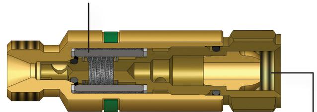
Reverse flow check valve prevents gas from backing up and mixing into the supply system. The valve is protected from damage by the sintered stainless steel flame trap.
